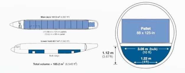
The B737-800BCF features main deck positions A1-A11 and K12, plus lower hold compartments. Weight limitations vary by position, ensuring optimal load distribution.
